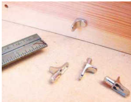
STEP 6. Calculate shelf positions so that spacing between them is uniform. Drill 5mm holes for the push-fit supports
